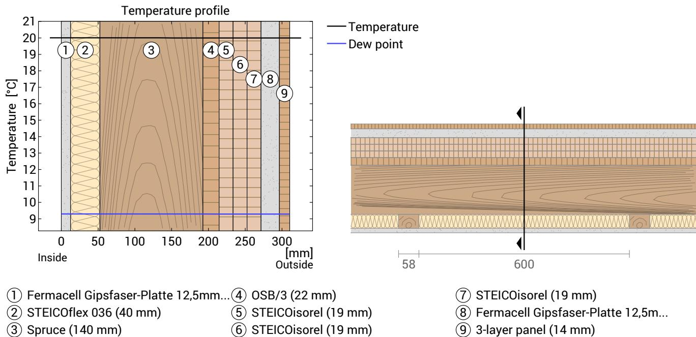
**Left:** Temperature and dew-point temperature at the place marked in the right figure. The dew-point indicates the temperature, at which water vapour condenses. As long as the temperature of the component is everywhere above the dew point, no condensation occurs. If the curves have contact, condensation occurs at the corresponding position.
