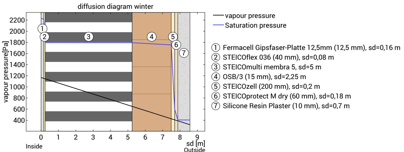
The section under investigation is free of condensate under the given climate conditions.
