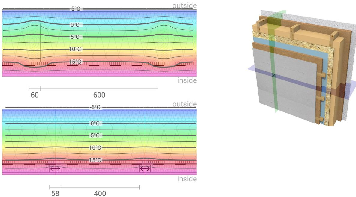
Top left: Temperature profile in the blue section (see right illustration). Bottom left: Temperature profile in the green section.
