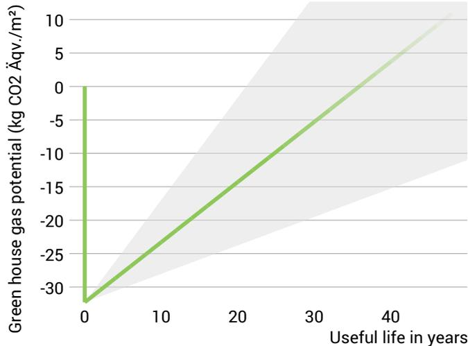
The **left figure** shows the global warming potential of the production of the component in the vertical part of the curve. Greenhouse gas emissions (through heating) arising during use of the building are indicated by the upward curve.
