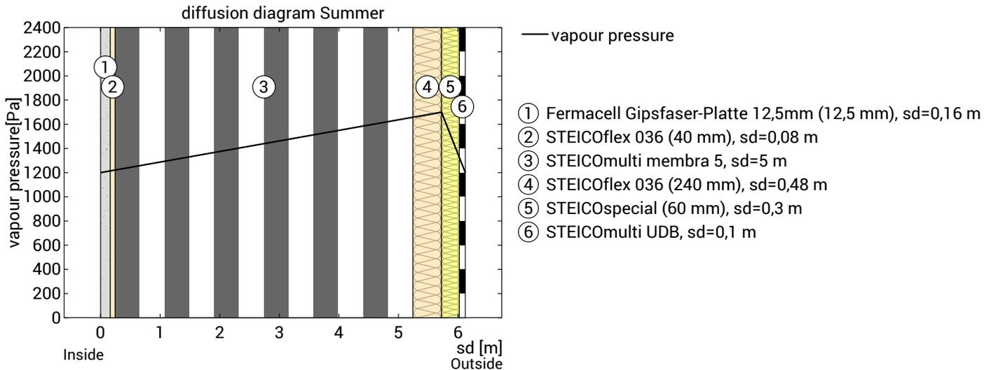
Condensate-free component: The maximum possible evaporation mass for the drying reserve is calculated. Consider the level that has the lowest evaporation potential in the dew period, at  $sd=5,72 \text{ m}$ ;  $x=29,3 \text{ cm}$ :
