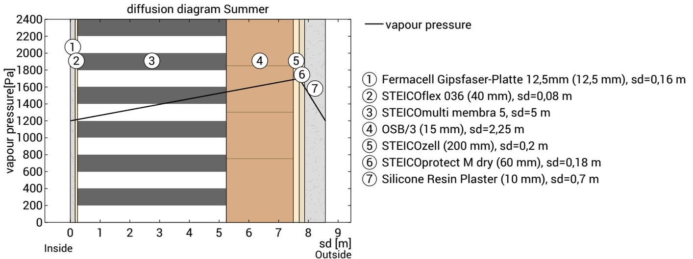
Condensate-free component: The maximum possible evaporation mass for the drying reserve is calculated. Consider the level that has the lowest evaporation potential in the dew period, at  $s_d=7,69 \text{ m}$ ;  $x=26,8 \text{ cm}$ :
