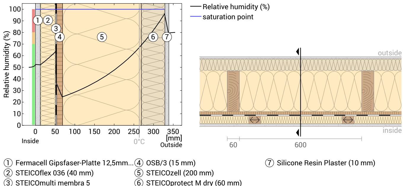
Layers marked with <-> run parallel to the illustrated cutting plane and were not taken into account in the moisture protection calculation.
