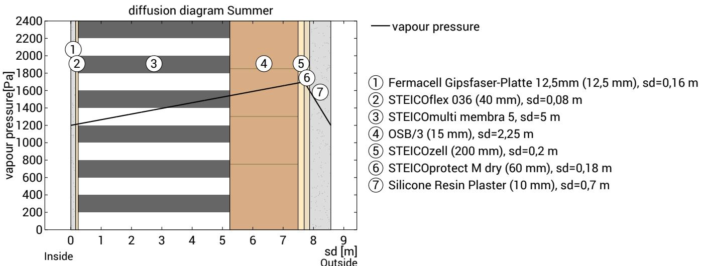
Condensate-free component: The maximum possible evaporation mass for the drying reserve is calculated. Consider the level that has the lowest evaporation potential in the dew period, at  $sd=7,69 \text{ m}; x=26,8 \text{ cm}$ :
